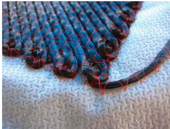
Abbildung 1: TFP-Darstellung. Quelle: https://www.compositesworld.com/articles/tailored-fiber-placement-besting-metal-in-volume-production
