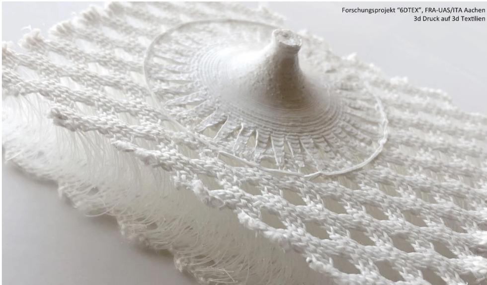
Figure 1: 3D printing on 3D textiles, project "6dTEX" FRA-UAS
