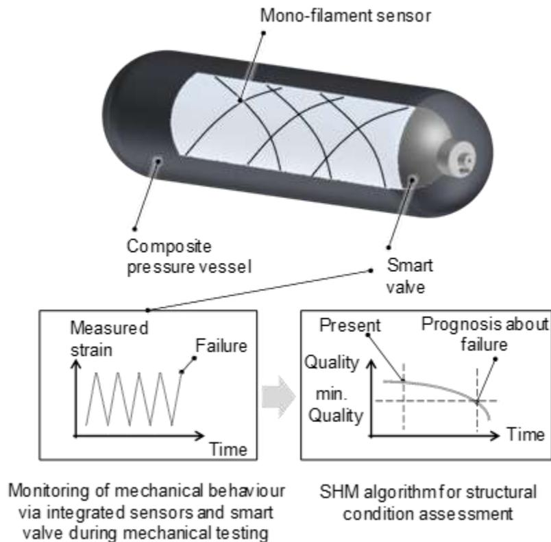
Fig.1: Concept for the instrumentation of composite pressure vessels for damage detection and condition assessment for hydrogen storage systems in mobile applications.
