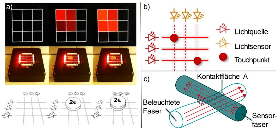
Figure 1: Pressure load measurement using cross-coupled polymer optical fibres (POF): a) Photo of 3x3 demonstrator, b) Schematic figure of 3x3 demonstrator, c) Principle of cross coupling.
