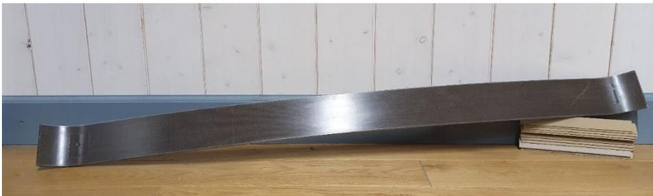
Abb.1: NFRP demonstrator of a leaf spring for a bogie of a narrow-gauge railway built by NOVACOM Verstärkte Kunststoffe GmbH, Aachen, Germany
