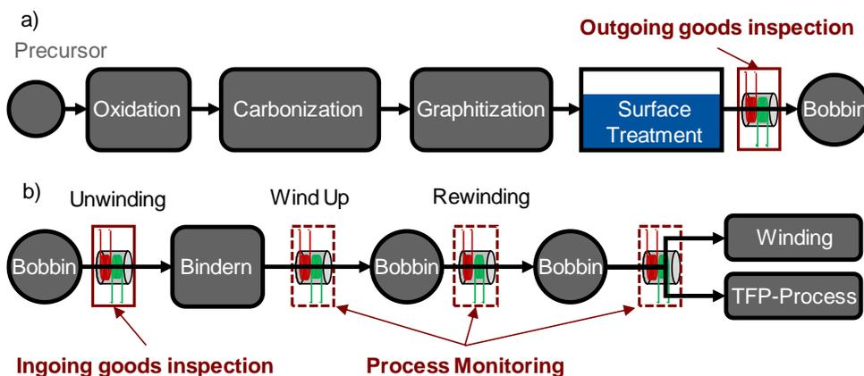
Figure 1: Application of the eddy current sensor in a) carbon fiber production and b) processing
