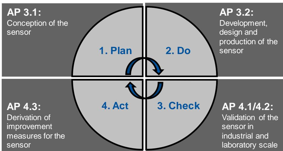
Figure 2: Deming cycle for the iterative development of the eddy current sensor
