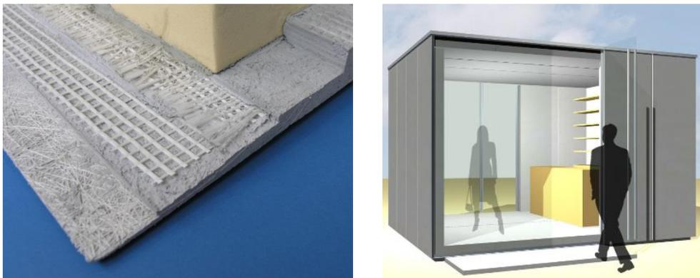
Figure 1: Textile-reinforced concrete (left); Café built in textile concrete modular design (right)
