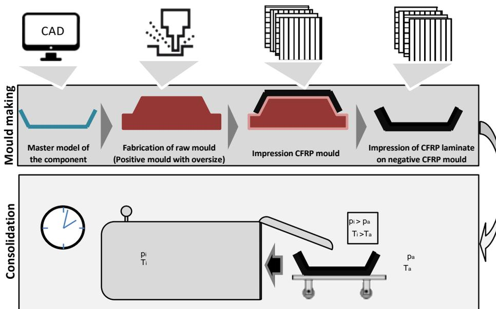
Figure 1: Process chain of mould making in the FRP component production
