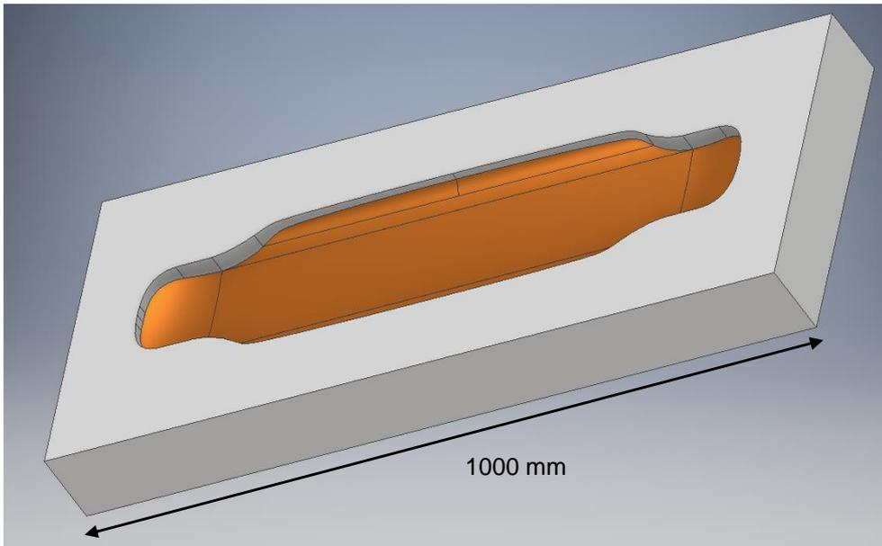
Figure 2: CAD model of the raw concrete mould as a negative mould
