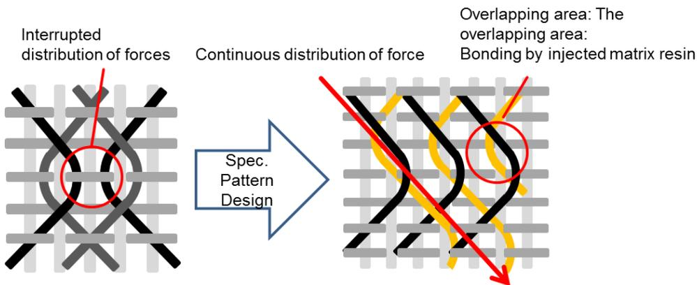
Figure 2: Principle of overlapping to generate the force transmission
