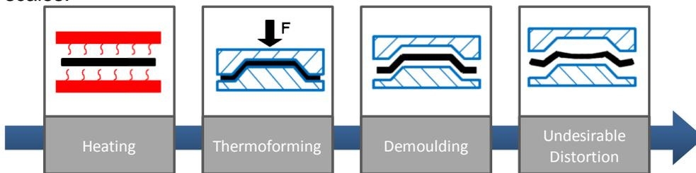
Figure 2: Steps in forming of a TPFRC sheet with frequently occurring shape distortions after deforming.
