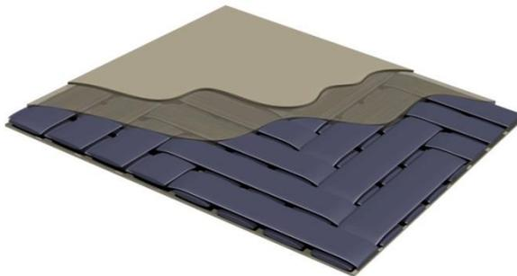
*Figure 1: Meso-scale schematic of TPFRC with one layer of 4x4 twill weave textile. The translucent layer represents the matrix infiltrating the textile. The opaque layer represents the outer neat TP matrix layer.*
