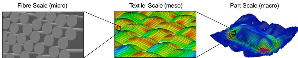
Figure 3: Three scales typical of a TPFRC: (left) micro, (middle) meso, and (right) macro.
