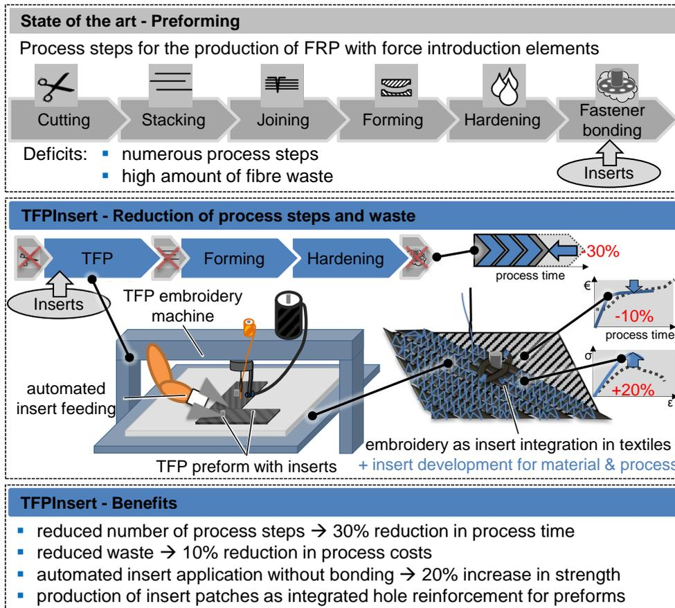
Figure 1: Central picture of the approach for the TFPInsert project
