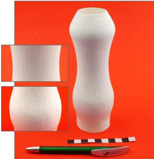
Fig. 1: OFC component manufactured using the freeze-casting process
