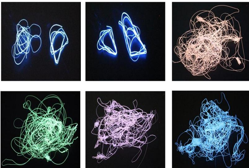
Yarns with different UV-active markers (wavelength 365 nm)
