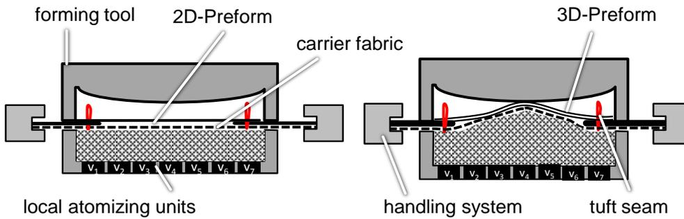
Fig. 1: Use of particle foam technology for forming preforms
