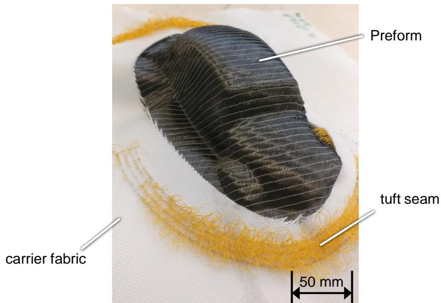
Fig. 2: Preform produced using tufting seam for material feed
