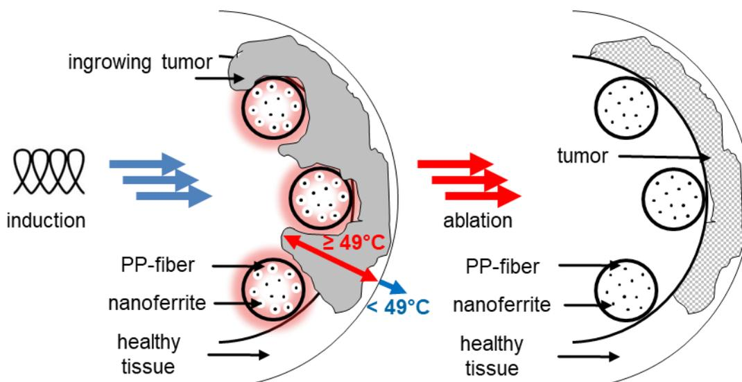
Figure 1 Nanoferrite-laden polymer fibers are inductively heated to locally destroy tumor tissue infiltrating a hollow organ through local hyperthermia.
